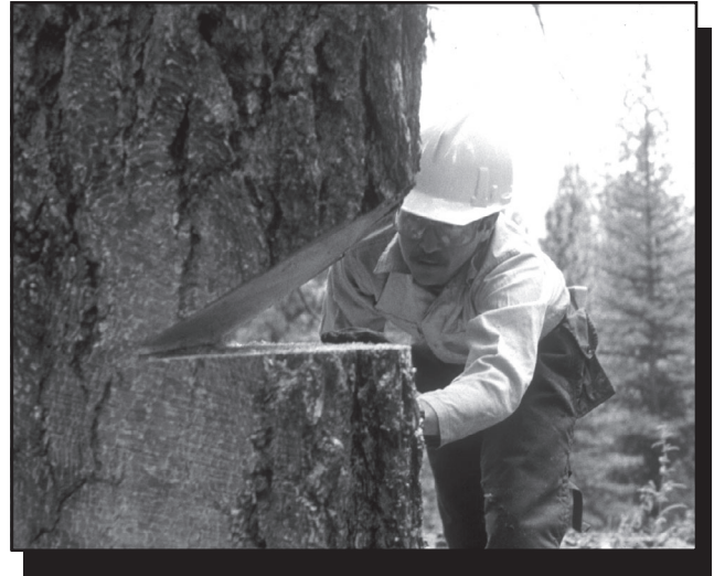
Figure 4-23—The sloping cut is a 45-degree angle.
