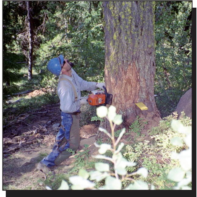
Figure 4-19—Complete the back cut.
